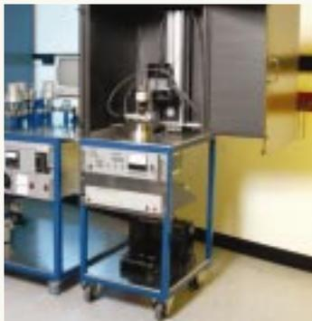
The Alphachron™ He Extraction/Measurement Instrument represents the latest development in (U-Th)/He technology. This is an automated, integrated and compact turnkey system, designed for the extraction and measurement of gases from mineral samples. The instrument is prefabricated and ready for implementation after delivery with minimal commissioning.
