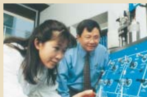
CSIRO Petroleum's Aileen Boudeville (left) and Dr Chee Tan (right) monitor mud filtrate flow rate in CSIRO's Membrane Efficiency Screening equipment.
