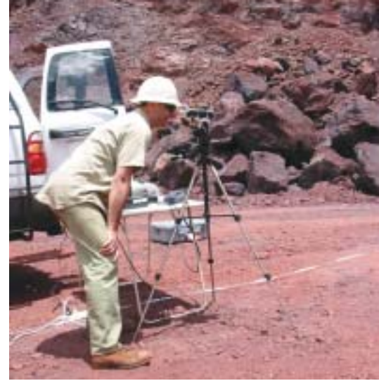
CSIRO's Erick Ramanaidou sets up the Spectral Mine Site System to use in field trials.
